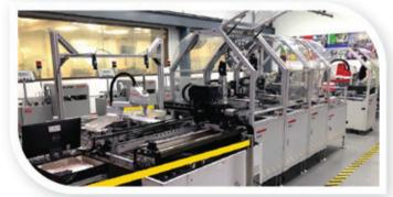
貿卡柔性生產線貫徹了「柔性生產製造單元」的概念,模組式的結構設計方便於生產工藝上的增 減和更換,該機採用的計算機輔助製造軟件(CAM),使換款時間縮短了75%。 The key of GF-450 is the term "Flexible"; module-design concept achieves the convenience of process modification needed for the different production. This machine is also supported by the computer aided manufacturing (CAM) software which can reduce 75% of the changeover time.
