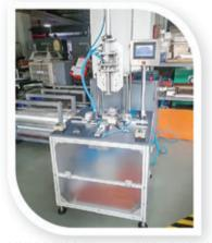
皮殼包邊機作為快速成型的項目,服務於集團主要產品之一一精 品盒;其通用性強的特點可以作為通用機型推廣給各分廠使用。 This four sides folding machine is used for pasting sheet paper onto the outside of cardboard box precisely and rapidly, It can be promoted as a general model, used for producing luxury packaging boxes which is one of the main products of the Group.
